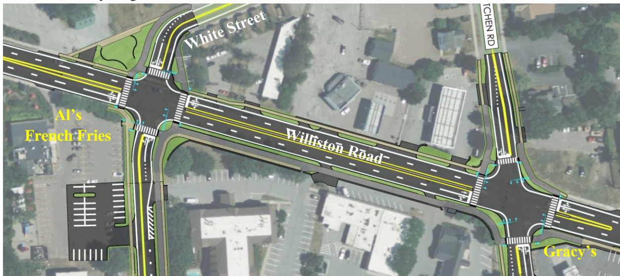
Figure 1: Illustration of the proposed realignment of the Williston Road White Street/Midas Drive intersection and the improvements to the Hinesburg Road/Patchen Road intersection with improvements between.
